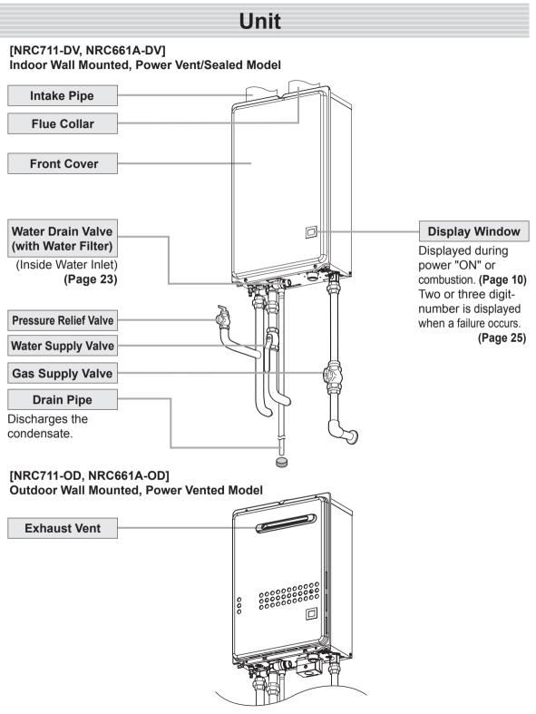
\* The above illustration shows an example of installation. The exact installation configuration may be slightly different.
