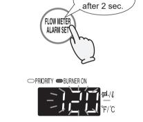
Change the temperature using the setting buttons.
